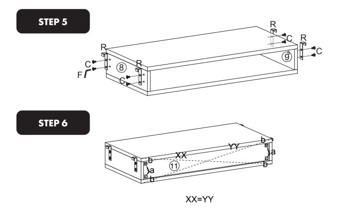
Ensure your Unit is square by measuring from corner to corner. If measurement for XX and YY are the same, then secure your Unit with Corner Brackets (b) and Screws (a).
