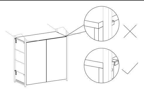
If required, adjust the positioning of the doors using the following steps:
