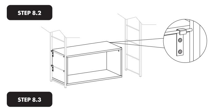
Ensure that the installed Unit is flush with the Ladder Frame.
