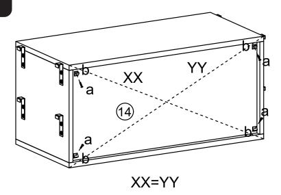
Ensure your Unit is square by measuring from corner to corner. If measurement for XX and YY are the same, then secure your Unit with Corner Brackets (b) and Screws (a).
